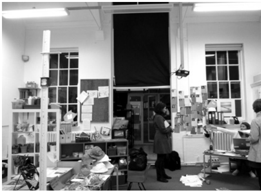
Above: Classroom before refurbishment - cluttered; windows fixed shut so no ventilation; blackout blinds to prevent over-heating meant lights were on all day.
